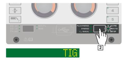
Press the "Welding process" button until the LED for the STICK/TIG welding process 2 lights up and "TIG" is shown on the display.
