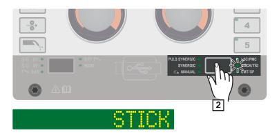
Press the "Welding process" button until the LED for the STICK/TIG welding process lights up and "STICK" is shown on the display.
