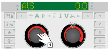
Parameter or entry from the Setup menu has been selected using the right adjusting dial; the LED on the right adjusting dial lights up.
